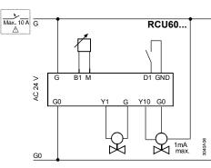
▲ For US installations, use Class 2 rated power supplies. For other installations, use circuit breakers with rated current of no more than 10 A.
