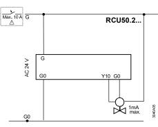
▲ For US installations, use Class 2 rated power supplies. For other installations, use circuit breakers with rated current of no more than 10 A.
